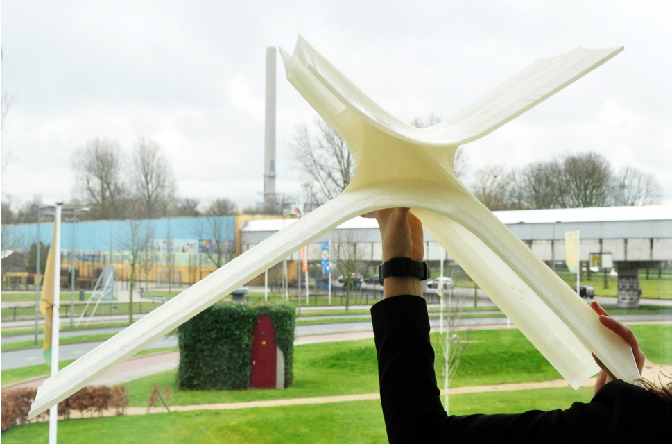
Figure 9: Physical prototype of a single shading element. Image and design by Ector Hoogstad Architecten & TU Delft
